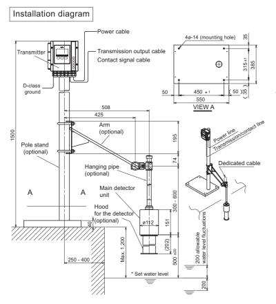
\* Set water level: The water level used when adjusting the optical axis; it will serve as a reference for determining the correct detectorls position and allowable water level fluctuation range.
